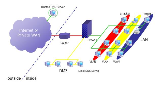
According to my test, a client's DNS cache can be effectively corrupted over VLANs. In this case, the predictability of the "Transaction ID" and the "UDP port number" opens/causes more severe problems to the security of the net.
