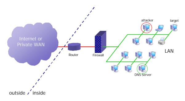
In this case, the DNS server, the target and the attacker are on the same net. So the attacker has to be quicker than the DNS Server. If we consider an application like dnspoison that cycles the transaction ID, for example, from 0 to 200, the chances to win the race are few. Other techniques, such as DNS Server flooding to try to slow it down, may help.
