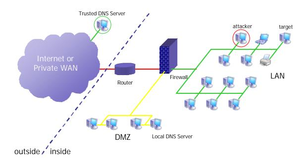
In this case the firewall introduces a delay in the packet dispatching, which, again, delays the DNS response.
